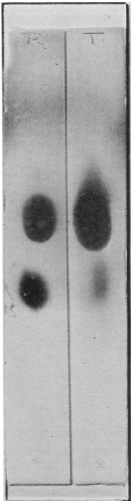
Fig. 1. Confirmation of identity of converted sulfoxide using thin layer chromatography. R, upper spot = chlorpromazine, lower spot = chlorpromazine sulfoxide. T, upper spot = converted product, lower spot = trace amounts sulfoxide.
